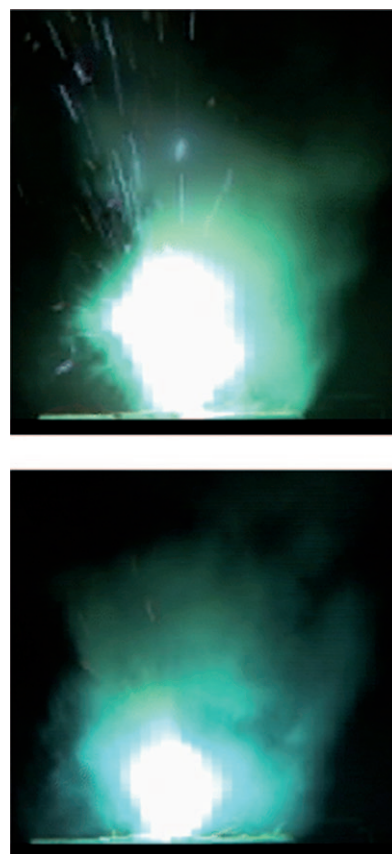
Figure 1. Photographs showing green-light emission of the M125 A1 control (top) and formulation G (bottom).
